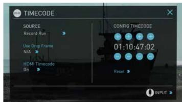
With this setting you set the starting Timecode for the first clip. The following clips will start at the frame immediately after the out point of the preceding clip. This will continue for all clips that follow. This is also known as continuous Timecode.
