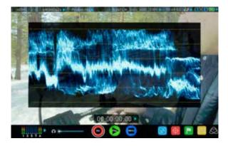
The Luma or Luminance Waveform is a great way to visualize the dynamic range of your image, allowing you to protect exposure of both your high lights and shadow detail. It's particularly useful when shooting with a low contrast LOG curve and works in perfect partnership with the AtomHDR engine to illustrate the highlight clipping point to allow you to correctly expose you image.
