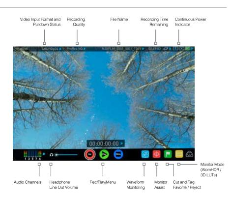
Touching the center of the screen at any time removes the top interface overlay, tapping again clears the bottom controls and a third tap brings all the options back up. Active Shot Setup or Monitor assist functions that are enabled will remain active when the menu system is cleared. This is to allow you to use the Shot Setup and Monitor assist functions at all times while shooting.
