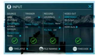
If HDMI timecode is selected and the camera is in REC RUN mode, the user has the choice to start and stop recording remotely from the source camera timecode.
