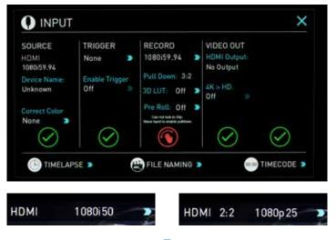
For these modes, simply press the > blue arrow underneath Record on the input menu repeatedly until your 1080p desired format is displayed. There is no need to wave your hand or the camera, as 2:2 pulldown removal does not require moving video.
