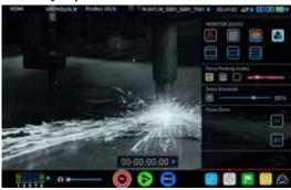
Blue only displays a greyscale image based on the blue channel of the input signal. This is useful to observe the noise content of a video image as sensor noise is most visible in this channel.
