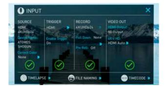
If the camera is Record Run mode, recording can be stopped or started by a moving Timecode via HDMI.
