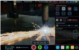
Zebra pattern show the parts of the image that are exposed +-5% of the target level set.
