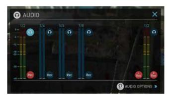
Each channel has a level meter assigned to Left & Right Channels; when there is active audio feed you will see the level indicator moving.
