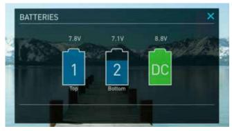
The Batteries screen indicator is made up of three icons, two will display the batteries and the other for the DC input. The active battery is shown in green and the level of the battery is shaded in 1/4 increments with a voltage level shown on top.
